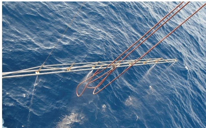
Spray nozzle manifold
